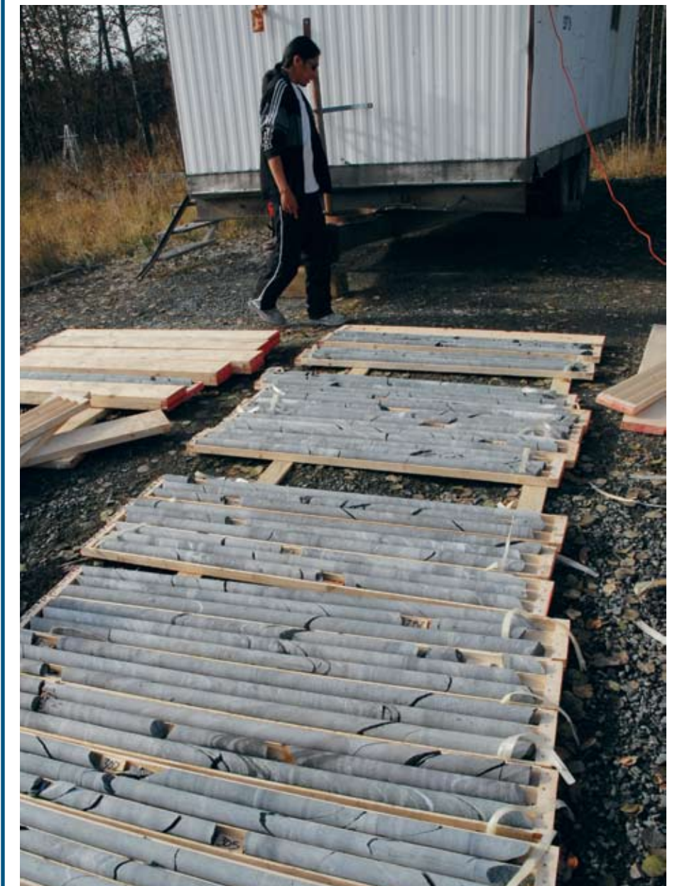
Top: A drilling company takes core samples to check for gold near Pickle Crow. Bottom: Ryan Neekan cuts core samples.
